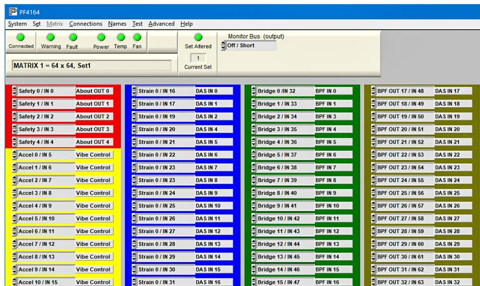
The Main GUI Section Screen with User-Defined Colored Coded Groups and Descriptive Channel Names
